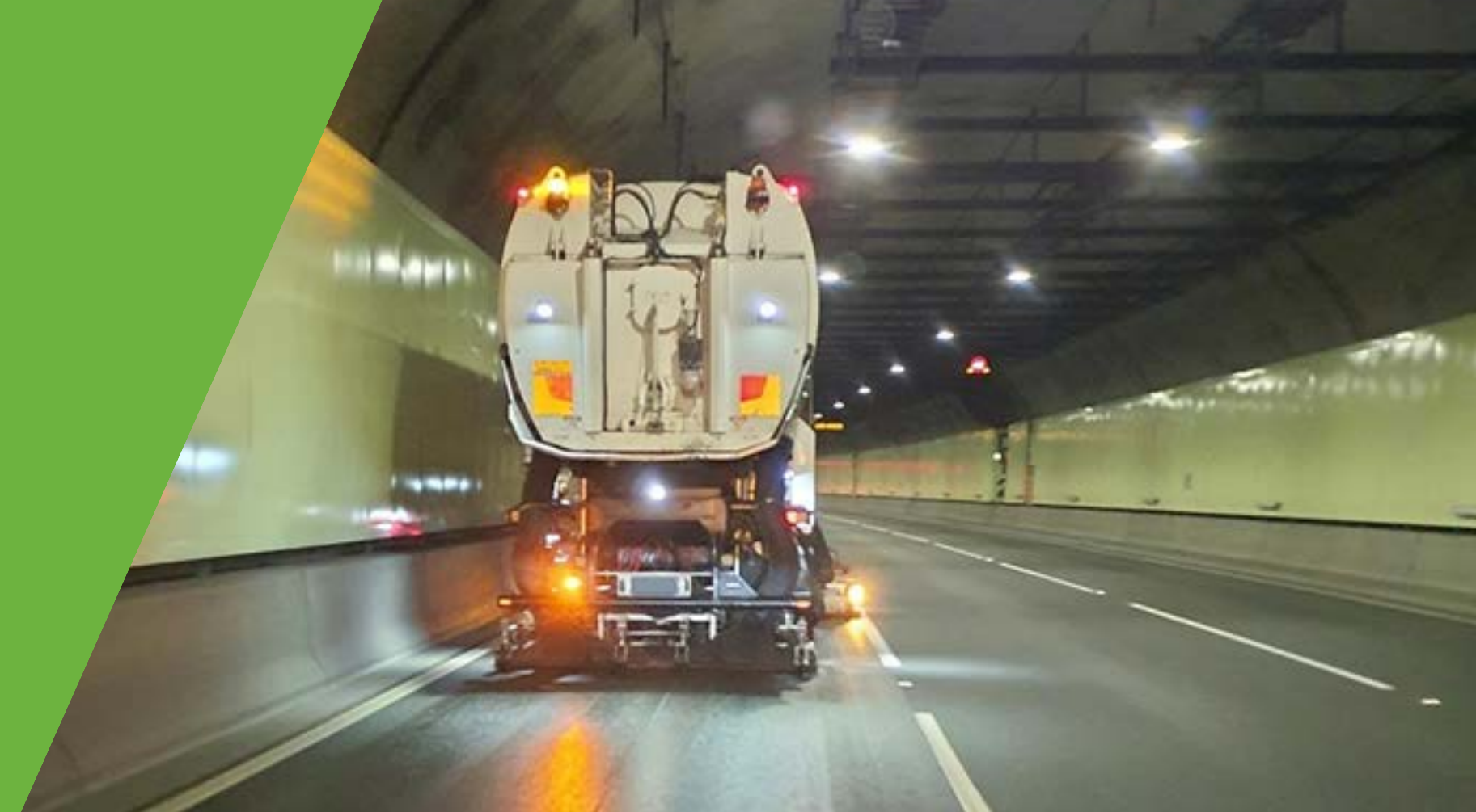
Heavy industrial cleaning trucks were brought down from Queensland to undertake a high pressure wash and clean of the tunnel pavement surface
