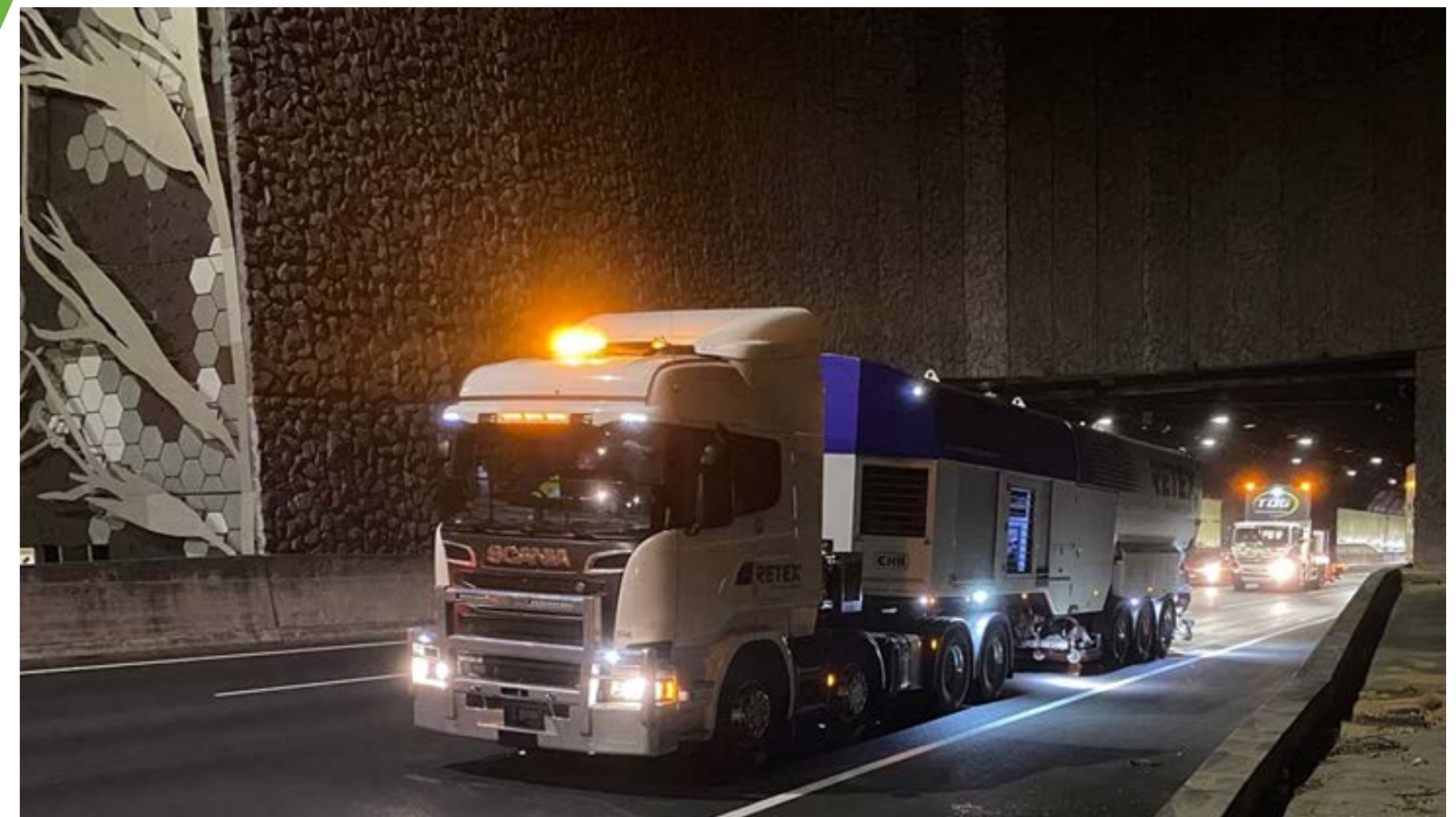
Heavy industrial cleaning trucks were brought down from Queensland to undertake a high pressure wash and clean of the tunnel pavement surface
